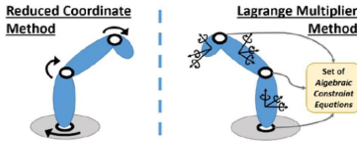
Figure 3: Overview of Multibody Dynamics Methods.
