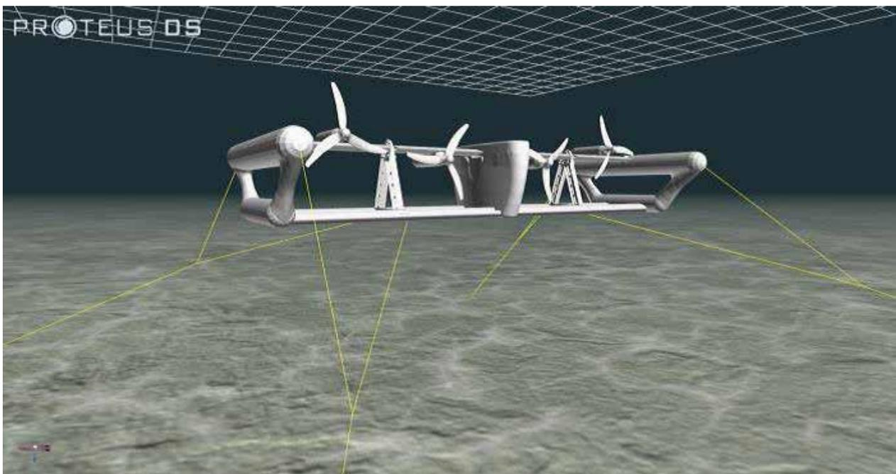
Figure 2: 3D visualisation of PLAT-O#2 platform and mooring lines [4]
